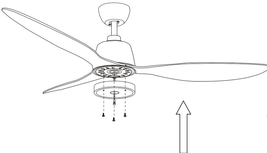
1. Remove three screws from the plate which on the motor.
