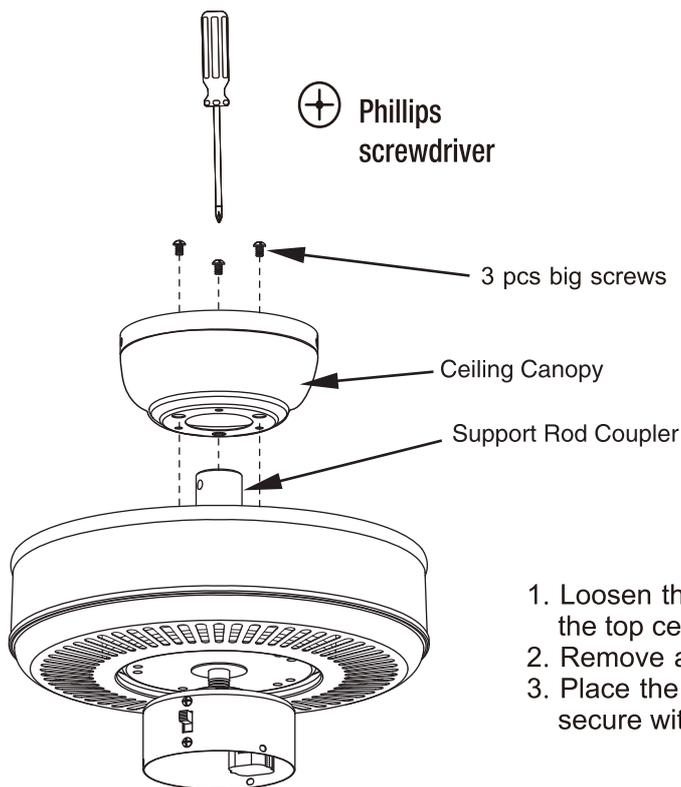
1. Loosen the set screws in the support rod coupler located on the top center of the motor housing until the inside channel is clear.
