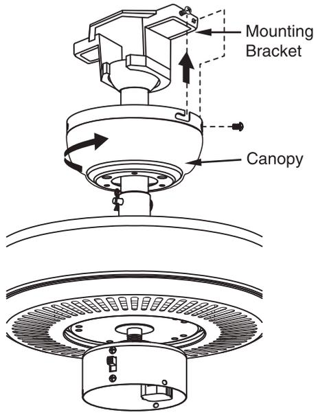
1. Notice the half ball on the end of the support rod is grooved down one side. This key way fits over the small keyway pin on the inside of the mounting bracket and keeps the ceiling fan from spinning on the mounting bracket.
