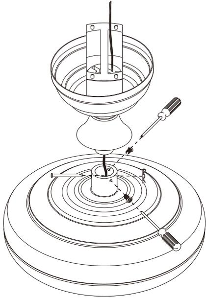
1. Thread the suspender through the suspended clock and coupling cover.
