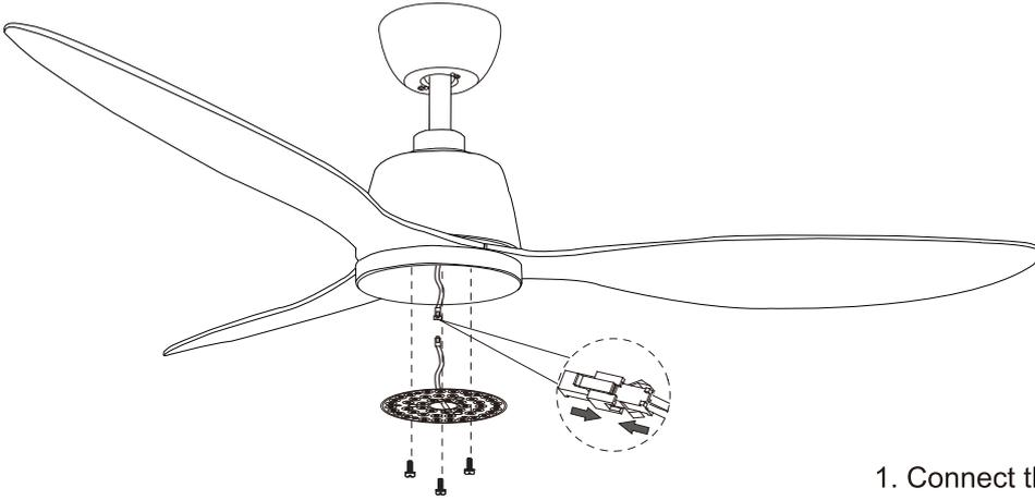
1. Connect the LED light kit to the motor.
