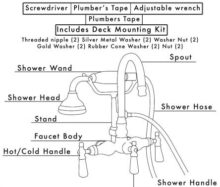
It is always advised to place plumber's tape on all threaded areas. 1. Assuming your water lines are prepared. Locate a threaded nipple, one silver metal washer, and a washer nut from the deck mounting kit. Slide the metal washer down the nipple and thread the washer nut onto the straight end of the nipple.
