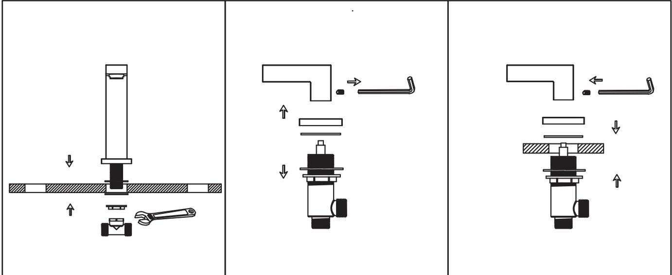
1. Remove the T-valve, lock nut and washer from the spout body. Place spout in center hole of sink. Assemble washer and tighten the lock nut to it. Connect the T-valve to the spout body using the wrench.
