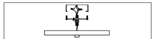
Step.4: Install fixture to bracket and tighten screws at the ends of the canopy (A) to secure.
