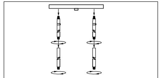
Step.2: Run wire through stems (B) and combine stem lengths to meet desired mounting height.
