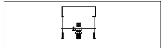
Step.1: Remove mounting bracket from fixture and install to electrical box
