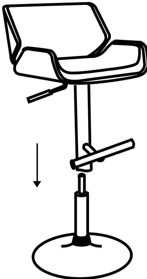
1. Place the assembled seat on Gas Lift (E).
