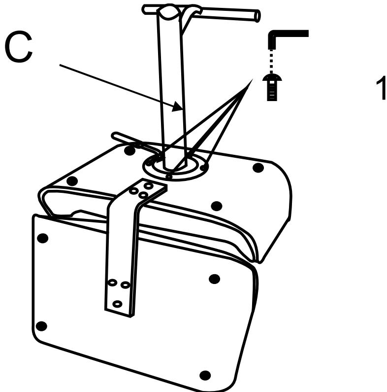
1. Place the attached Back and Seat upside down on a flat, smooth surface.
