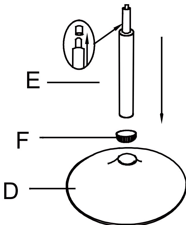
1. Remove the cap from the Gas Lift (E).
