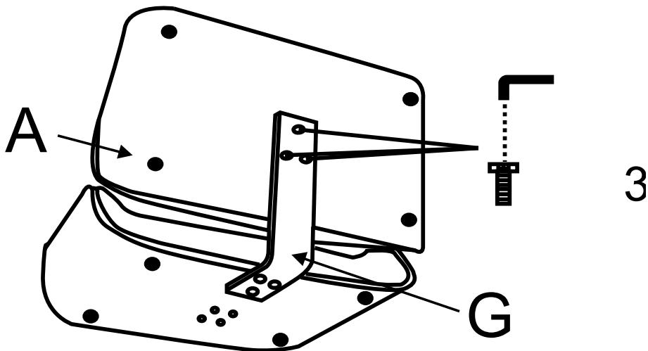
1. Attach Back (A) to Connector (G) using Allen Key Screws (3).
