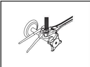
(4) Use faucet inlet supply hose to connect to supply stop. You may need adapter(not included) if supply stop outlet size is not 3/8" compression.
