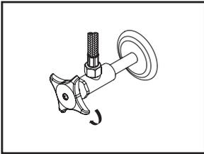
(1) Shut off water supply. Remove old faucet. Clean mounting surface in preparation for new faucet.
