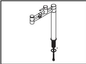
(2) Do not remove plastic arm bracket before finish installation to prevent damage on swivel arms. Be sure to place gasket underneath of faucet to form watertight seal.
