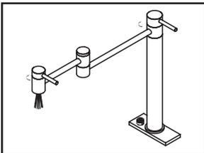
(6) Remove the aerator from the spout by turning counter-clockwise. Turn on supply stop. Check of any leaks. Make sure all the connection are secure. Open both handles. Flush and allow water to run at full flow for at least one minute. Turn off water. Replace the aerator.
