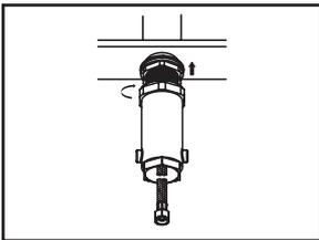
(3) Guide the faucet through mounting hole. Slide the washer from beneath the mounting surface. Install the locknut with the help of mounting tool
