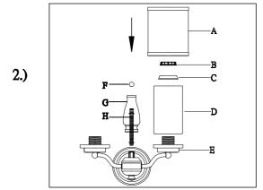
Step.2: Place shade (A) over socket. Attach glass (D) to fixture using socket ring (B) and spacer (C) to secure. Add medium base bulbs.
