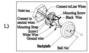
Step.1: Remove mounting strap from fixture and install to electrical box. Wire fixture to wires in outlet box. Copper wire is for Ground. Attach back plate to mounting strap and tighten ball nuts so fixture meets wall.
