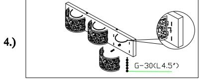
Step. 4: Slide shade (H) onto clips, install G9 bulbs (F) and hang crystal strands (G).
