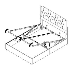
To avoid deformation of the metal frame, do not operate from the sides of the bed.
