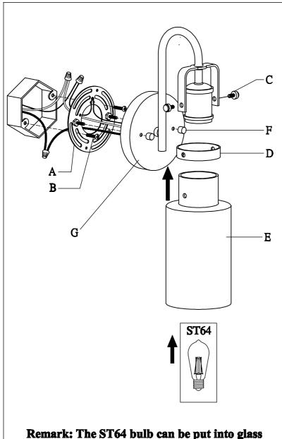
Step.1:Remove mounting bracket (A) from fixture and install to electrical box.
