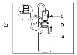
Step.2: Attach metal ring (D) and glass (E) to yoke and secure using set screws(C).
