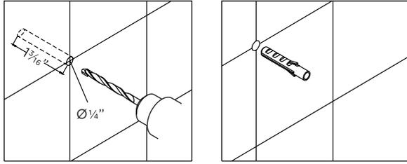
1. Using a 1/4" drill bit, drill two pilot holes approximately 1-3/16 " deep and use the base bracket to determine the distance apart.
