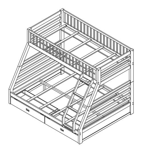
**IMPORTANT**: Do not tighten bolts completely until all bolt are completely lined up and inserted into holes
