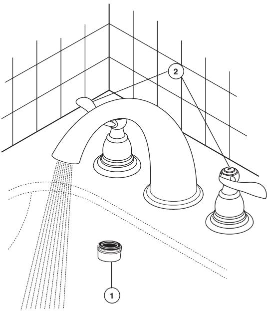
Remove Stream Straightener (1), turn faucet handles (2) all the way on. Turn on hot and cold water supplies and flush water lines for one minute.
