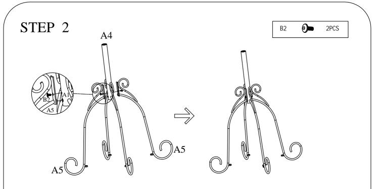
Attach the legs A5 to the bottom pole A4 using bolts B2. Please do not tighten bolts B2 until step 4.
