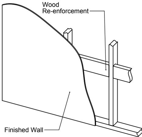
**2** Measuring for the desired height, secure all four wall brackets (B) to the wall. Make sure that screws (C) go into the re-enforced area of the wall. 29.5" to the top screw is the recommended height.
