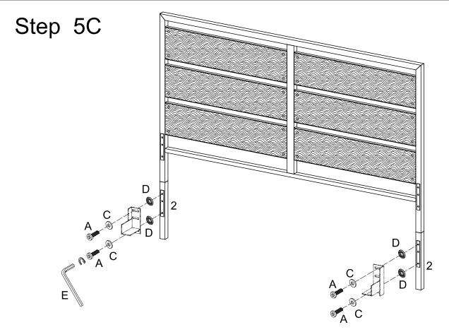
Use wrench (E) to secure bed rail (not included) to leg (2) with bolt (A), washer (C) and washer (D).
