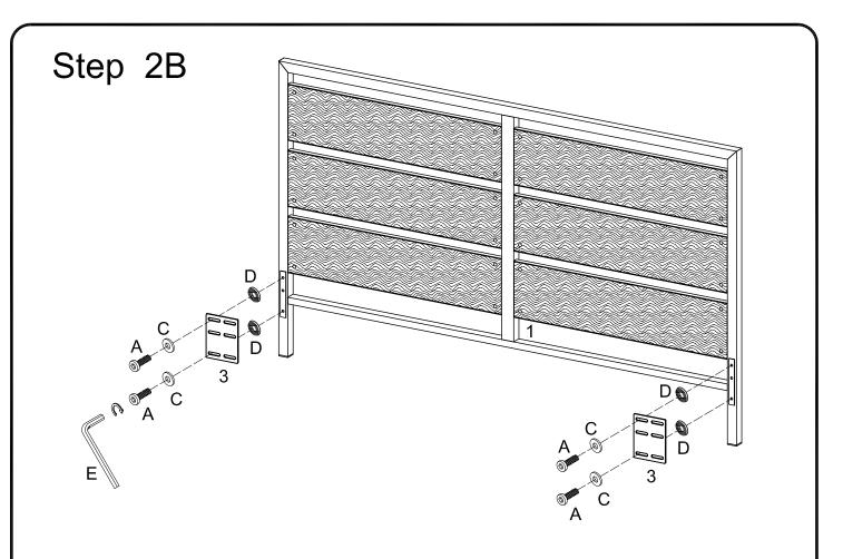
Use wrench (E) to secure plate (3) to head board (1) with bolt (A), washer (C) and washer (D).
