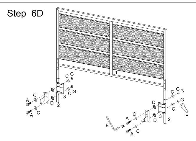
Use wrench (E) to secure bed rail (not included) to plate (3) and leg (2) with bolt (A), washer (C), washer (D) and secure nut (G) by using wrench (F).
