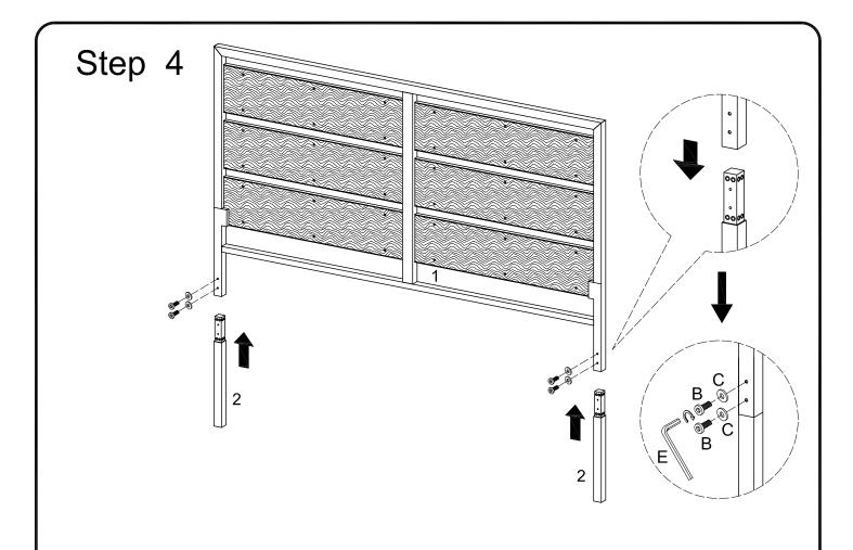
Insert leg (2) into head board (1), use wrench (E) to secure it with bolt (B), washer (C).
