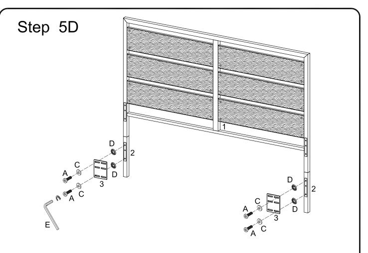
Use wrench (E) to secure plate (3) to leg (2) with bolt (A), washer (C) and washer (D).
