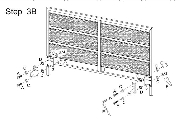
Use wrench (E) to secure bed rail (not included) to plate (3) and head board (1) with bolt (A), washer (C), washer (D) and secure nut (G) by using wrench (F).
