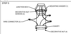
Install the recommended bulb in the socket, and then install the canopy (shade/cover) of the decorative fixture to the mounting hanger, using the supplied screws or decorative nuts (4).
