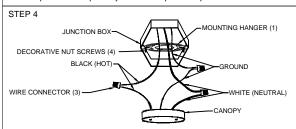
Connect the hot wire from main wire to the hot wire from power supply. Connect the neutral wire from the main wire to the neutral wire from power supply. Fix the ground wire from fitting to ground wire(grounding) from power supply.
