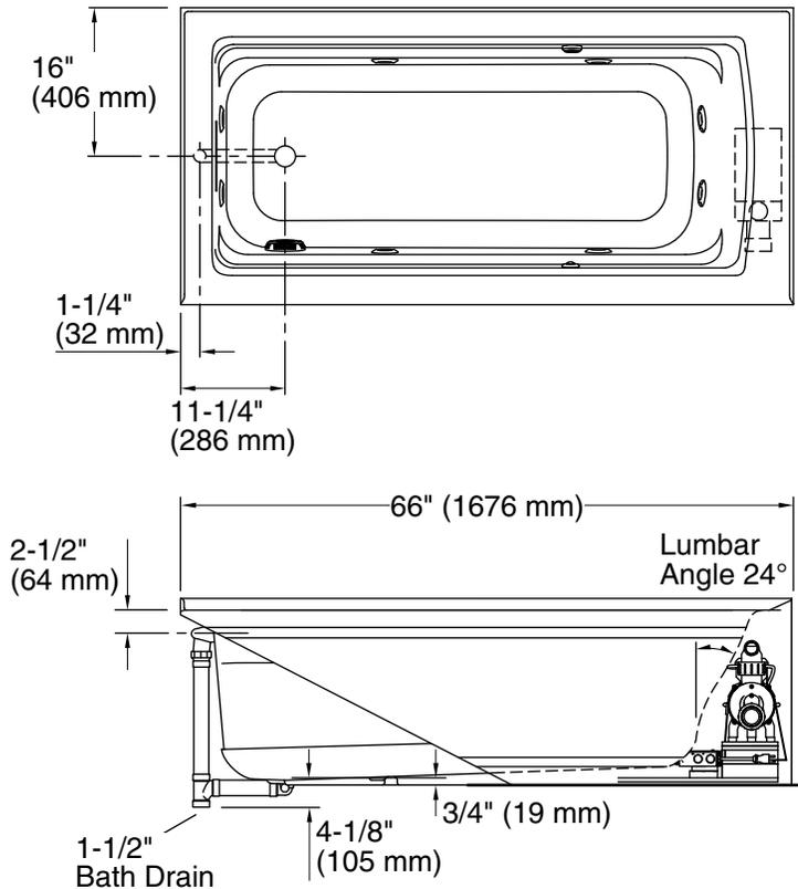
No change in measurements if connected with drain illustrated. (K-7272)
