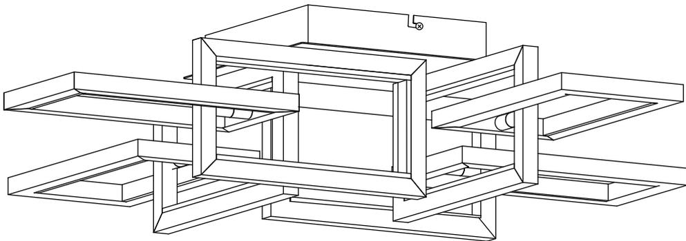
This fixture is designed to dim with an Electronic Low Voltage dimmer. Dimming levels will vary by dimmer.
