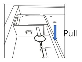
STEP 3. – Push the same pins into position to locked the four legs after straight.
