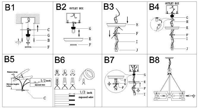
Step B1: Remove the threaded ring (F) from collar loop(G). Attach the single bar (C) to outlet box with mounting screws (B). The side of single bar marked "GND" must face out ,Unscrew the collar ring (H) from the collar loop.
