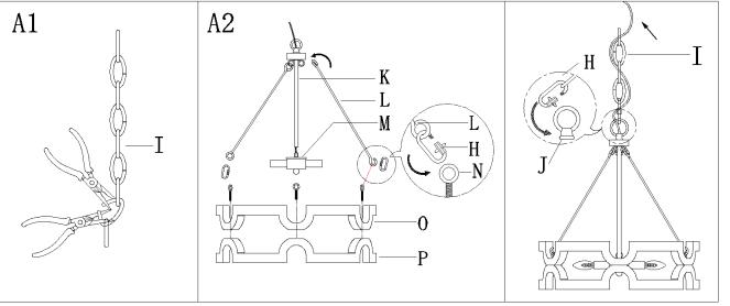
Step A1: By measuring, determine the correct number of links needed for proper hanging height. Using the chain pliers, disconnect and discard the remaining chain.
