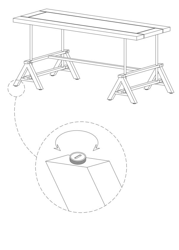
Note: Levelers on bottom of legs can be adjusted if floor is uneven.
