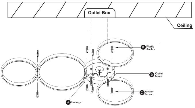
Attach canopy (A) to outlet box with outlet screws (D). Screw anchor screws (C) into plastic anchors (B) to secure canopy (A).
