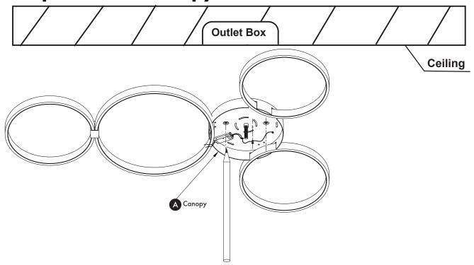
Remove canopy cover from canopy (A). Raise canopy (A) to the ceiling. Mark location for plastic anchors (B). Drill holes for plastic anchors (B). Insert plastic anchors (B) into hole.
