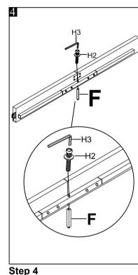
Attach support legs "F" to wood bar "K" .Using Allen key (H3) to lock with bolts "H2".
