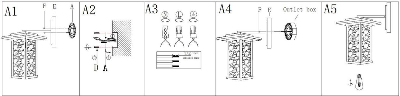
Step A1: Unscrew the knob nut(F) from back plate(E) then gently remove mounting plate (A)
