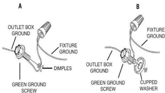
Connect wires according to below chart
