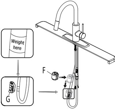
Install the weight clip (G) at the point of the hose marking "weight here". Insert the weight (F) onto the weight clip (G) by sliding it down onto the weight clip (G).
