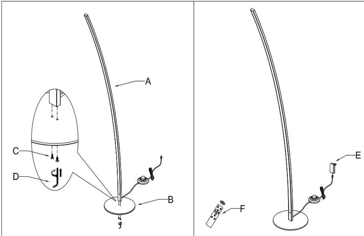
1.Locking main body stents (A) to counter weight (B) with screw (C) and allen wrench(D).
