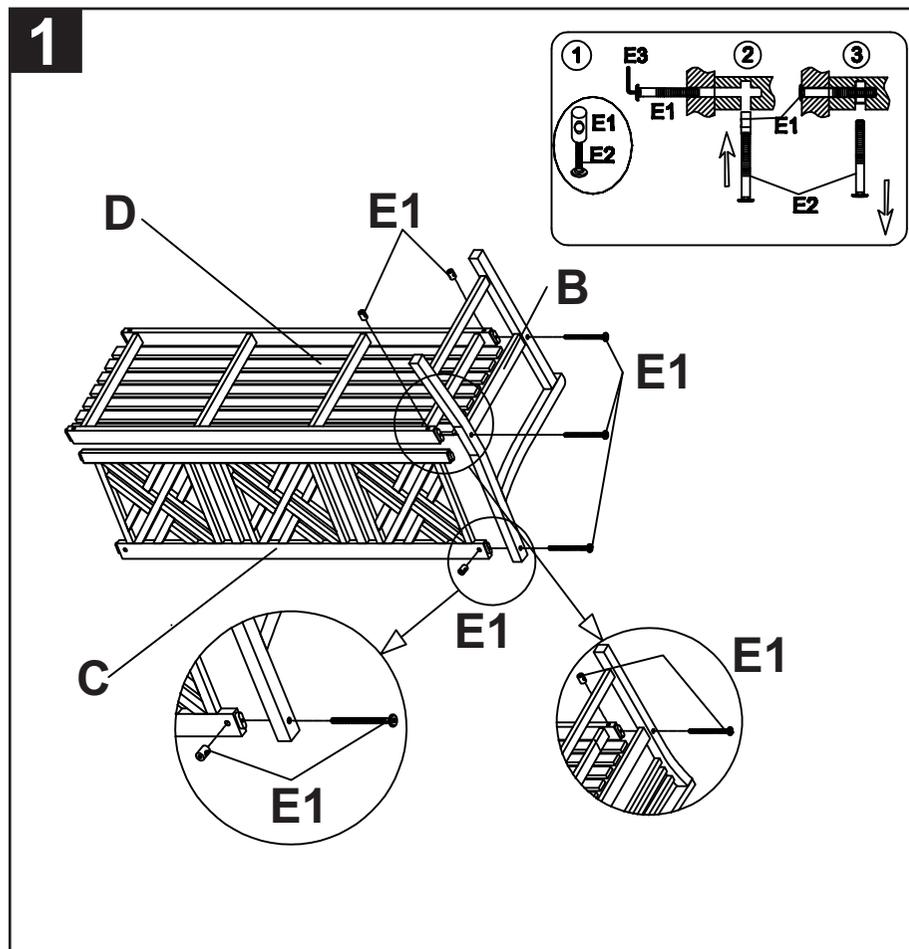
Step 1: attach the left side (B) to the back (C) and the seat (D) as shown on the picture by using the Allen bolt (E1). Tighten all with the Allen key (E3).
