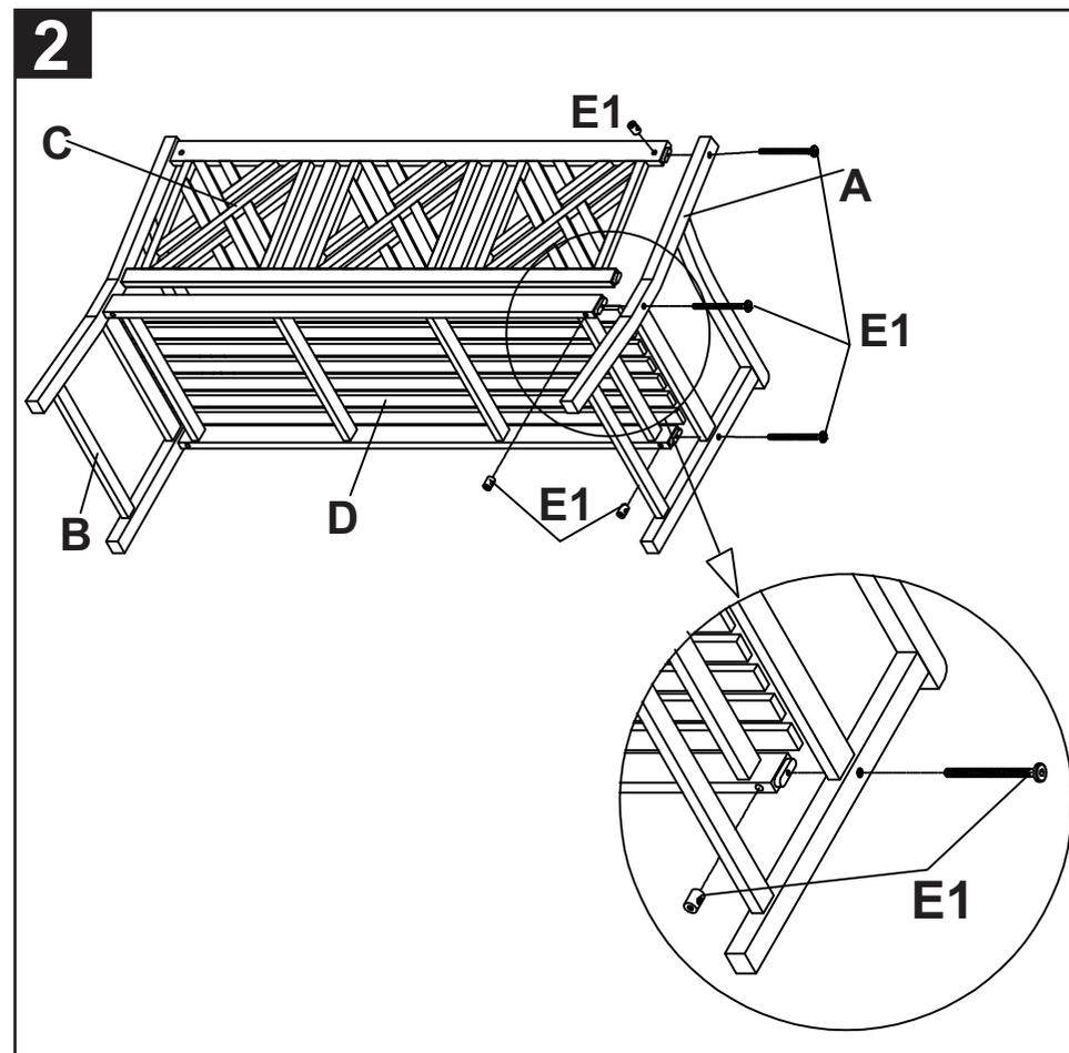
Step 2: attach the right side (A) to the bench as shown on the picture. Repeat the right side (A) in the same way as step 1.
