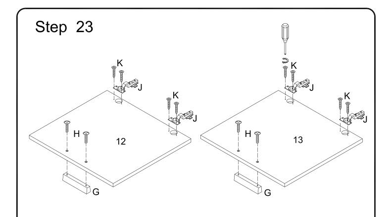
Attach hinge (J) to doors (12,13) using screws (K). Attach handles (G) using bolts (H).
