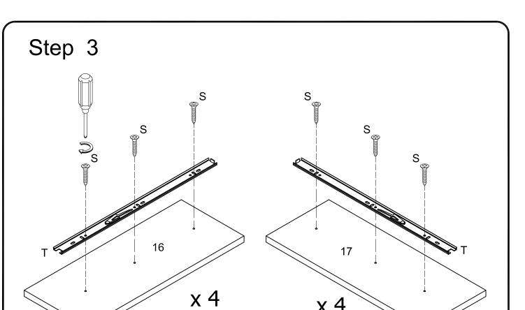
Secure screw (S) to the tray bracket of keyboard tray slider (T) to the drawer side panel (16,17).
