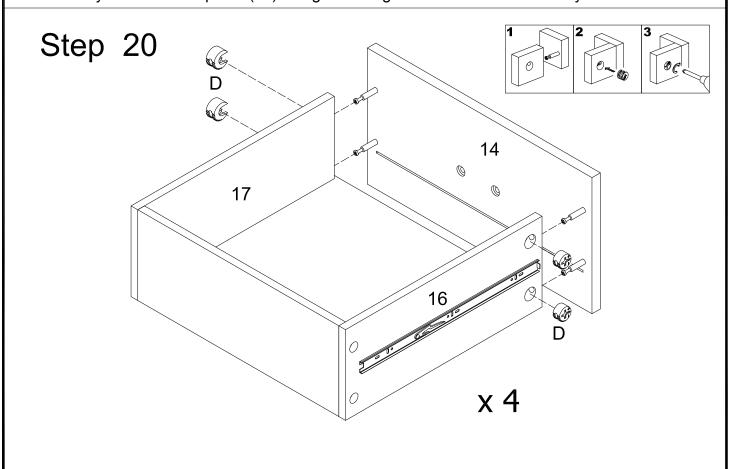
Attach door panel (14) to assembled drawer using cam locks (D).
