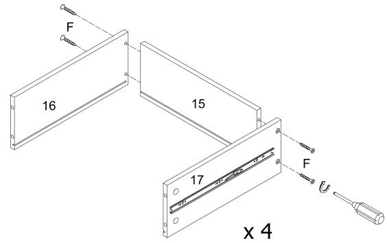
Attach drawer panels (16,17) to drawer panel (15) using screws (F).
