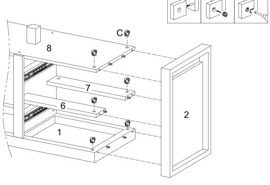
Attach side panel (2) to unit using cam locks (C).
