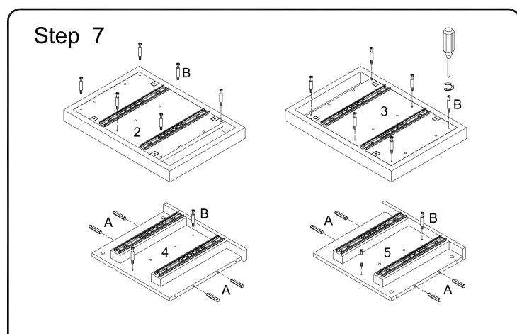
Secure cam bolts (B) into panels (2,3,4,5). Insert wooden dowels (A) into panels (4,5).
