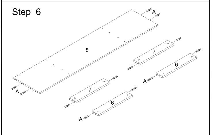
Insert wooden dowels (A) into bottom panel (8) and support bars (6,7).
