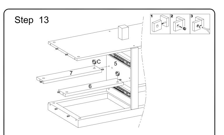
Attach support bars (6,7) to side panel (5) using cam locks (C).
