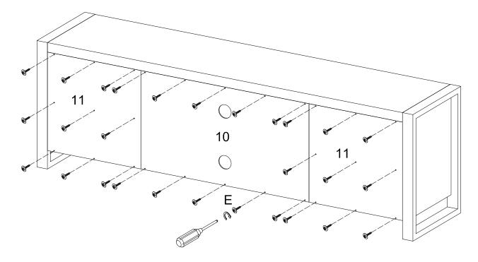
Attach back panels (10,11) to unit using screws (E).
