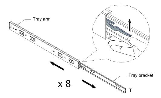
Disassemble keyboard tray slider (T) by sliding the tray arm and tray bracket apart. Depress the small lever of the tray bracket and carefully pull the two pieces apart. Repeat this process for both keyboard tray sliders (T).
