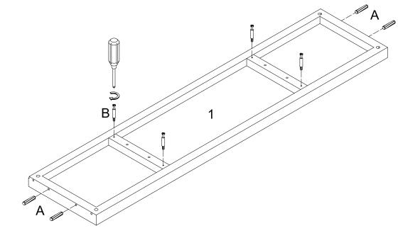
Secure cam bolts (B) and insert wooden dowels (A) into top panel (1).
