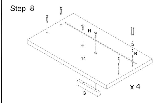
Attach drawer handle (G) using bolts (H) and secure cam bolts (B) into drawer panels (14).
