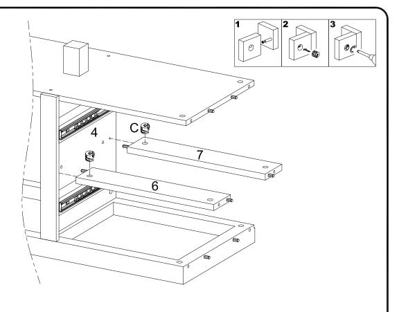
Attach support bars (6,7) to side panel (4) using cam locks (C).
