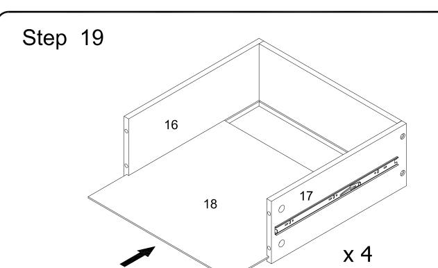
Carefully insert drawer panel (18) along the thin grooves of drawer assembly.
