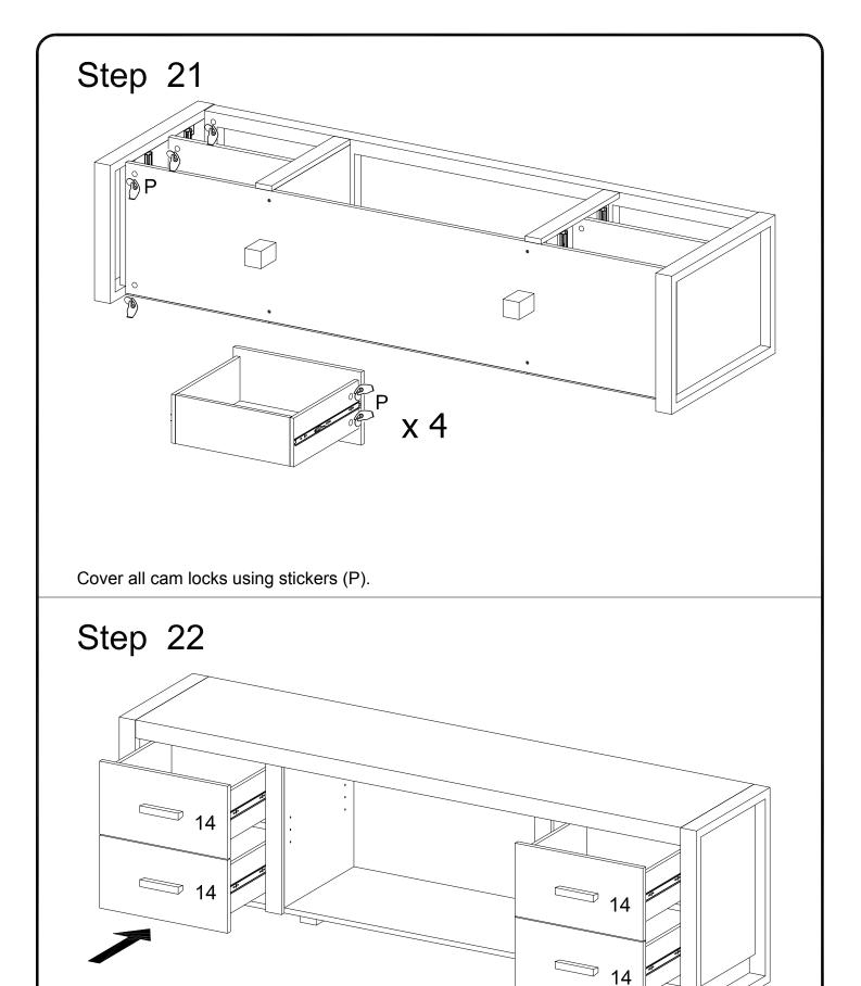
Carefully insert drawer assembly into assembled unit.
