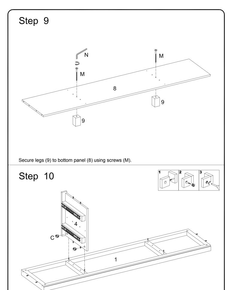
Attach side panel (4) to top panel (1) using cam locks (C).
