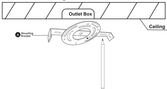
Raise mounting bracket (A) to the ceiling. Mark location for the plastic anchors (B). Drill holes for plastic anchors (B). Insert plastic anchors (B) into hole.
