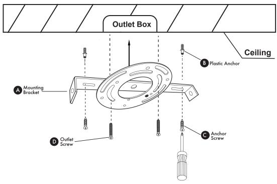
Attach mounting bracket (A) to outlet box with outlet screws (D). Screw anchor screws (C) into plastic anchors (B) to secure mounting bracket (A).
