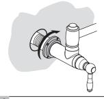
Remove the faucet from the supply pipe. Remove the mounting plate from the shank.
