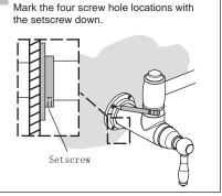
Install a 1/2" NPT supply pipe to extend no more than 1/2" (13mm) beyond the wall.
