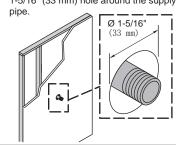
Thread the shank to the supply pipe so the mounting plate is flush.
