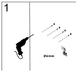
For drywall installation, mark the hole locations and drill Φ 6mm holes for the drywall anchors. Install a junction box behind the mirror for power connections.
