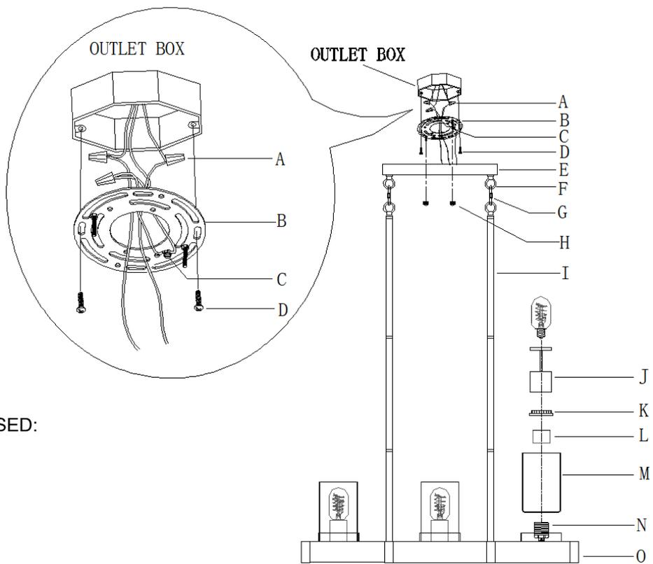
3. According your desired hanging length to select and use the tubes (I) then pass the wires through the tubes(I) to the top of loop .Gently pull wires and thread the tubes (I)onto the fixture (O) till tight
