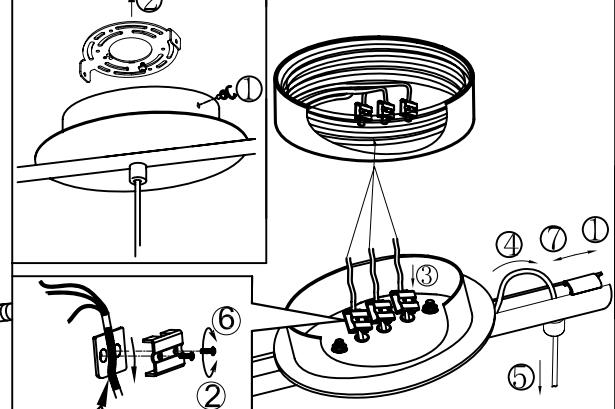
Always keep the fiberglass sleeving between the metal strain relief and the cord to protect the cord from damage
