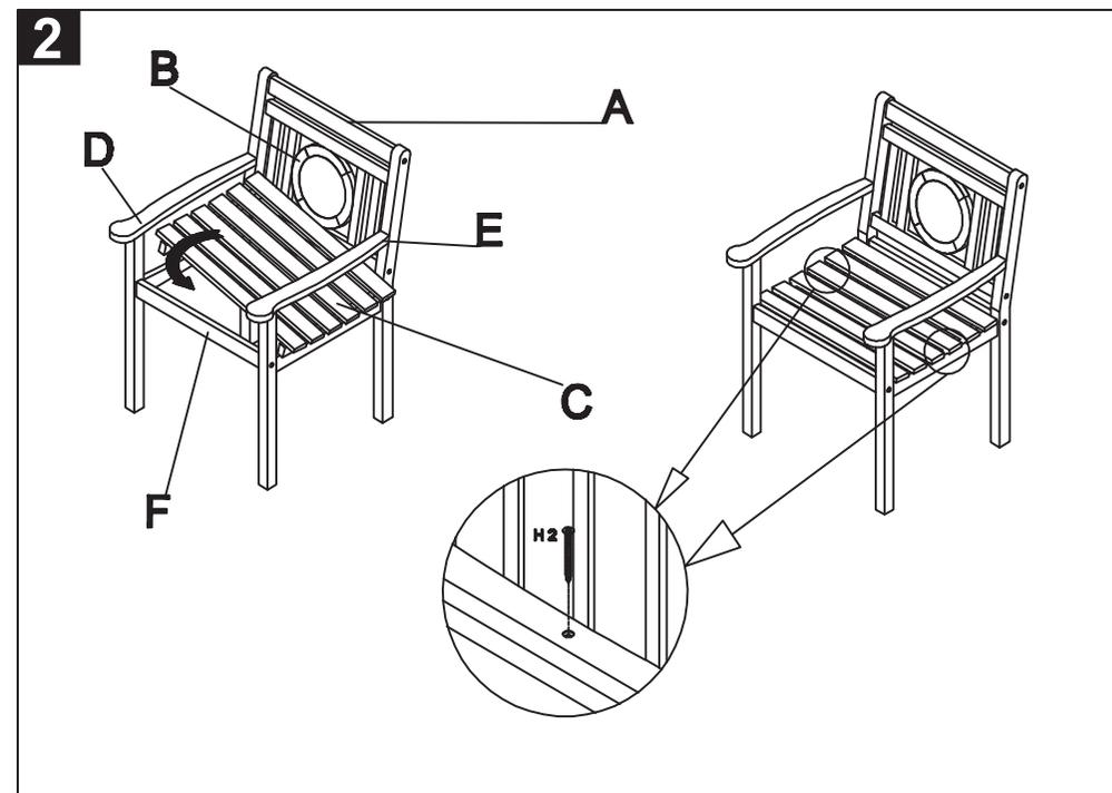
Step 1: attach left side (E) to back (B) with support 1 (A) and support 2 (F) as shown on picture,using bolt (H1) and tighten with the Allen key (H4) .
