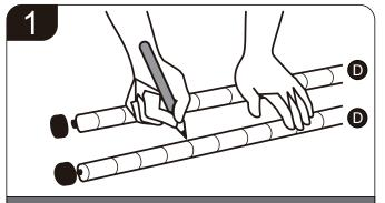
Use a pen to mark the height on the 4 Lower Poles (D). Be sure all poles are marked in the same location.
