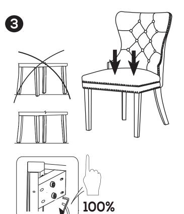
Put chair in the upright position and SIT ON THE CHAIR to press downwards on the seat pad ensuring that all 4 feet touch the ground and chair is leveled.
