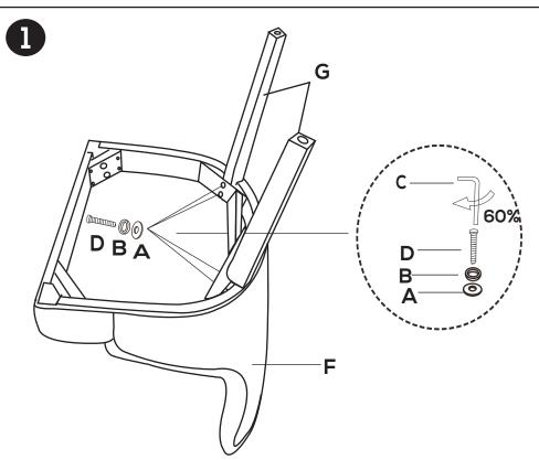
Put chair back on a clean flat surface. Align Hind legs in the seat pad as shown in the diagram.
