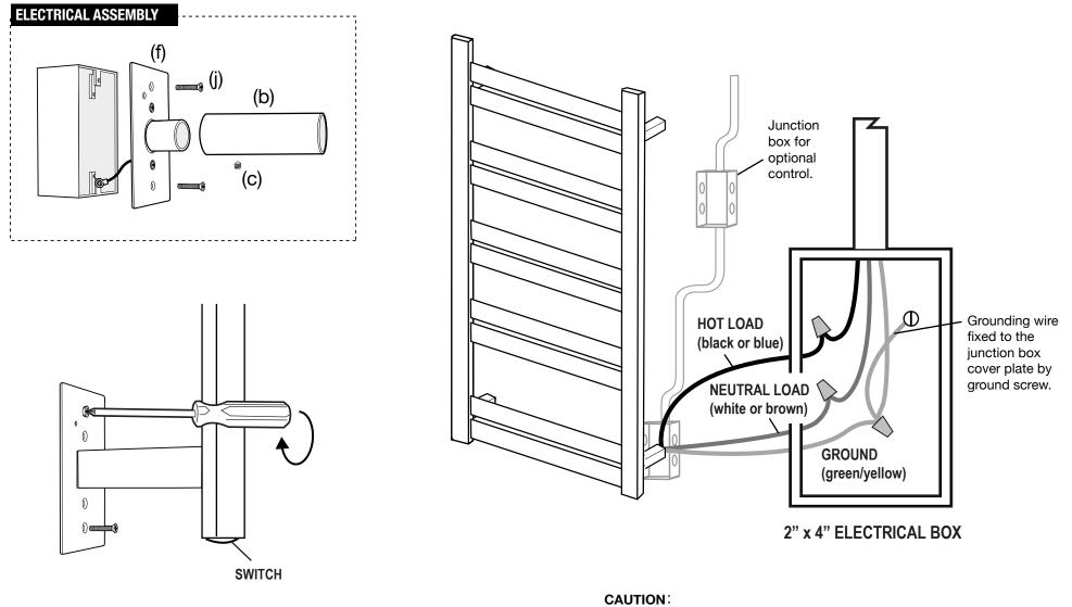
To provide continued protection against risk of electric shock, connect to properly grounded outlets only.
