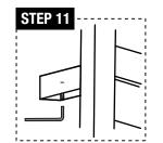
**STEP 11:** As shown in the picture, install the set screws (c) into the hole of all the tubes (a and b) using the allen wrench; fix the tube (a) onto the mounting bracket (g).
