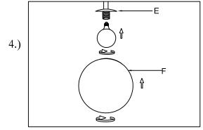
Step 4: Install 60 Watts medium base bulb . Then install glass (F) into cup (E).
