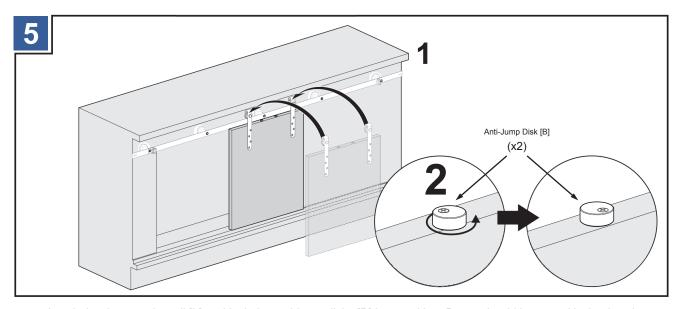
Attach the doors to the rail [L] and lock the anti-jump disks [B] into position. Doors should be routed beforehand if using the routed door guide [G].
