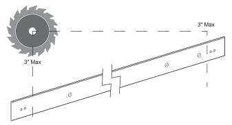
The rail can be trimmed if necessary using a band saw. Use blades suitable for iron or stainless steel depending on your rail.
