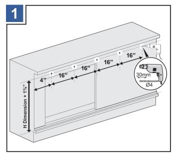
Using a power drill with a 4mm drill bit, drill holes as indicated.
