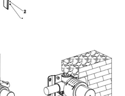
2. Put the protective cover on the valve body and finish the
