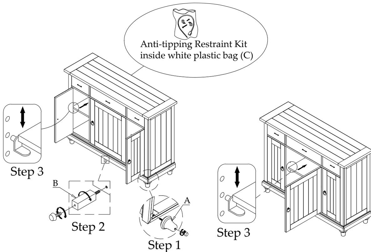
Step 1: Place the Server on its back. Attach a Bun Foot (A) at each corner.
