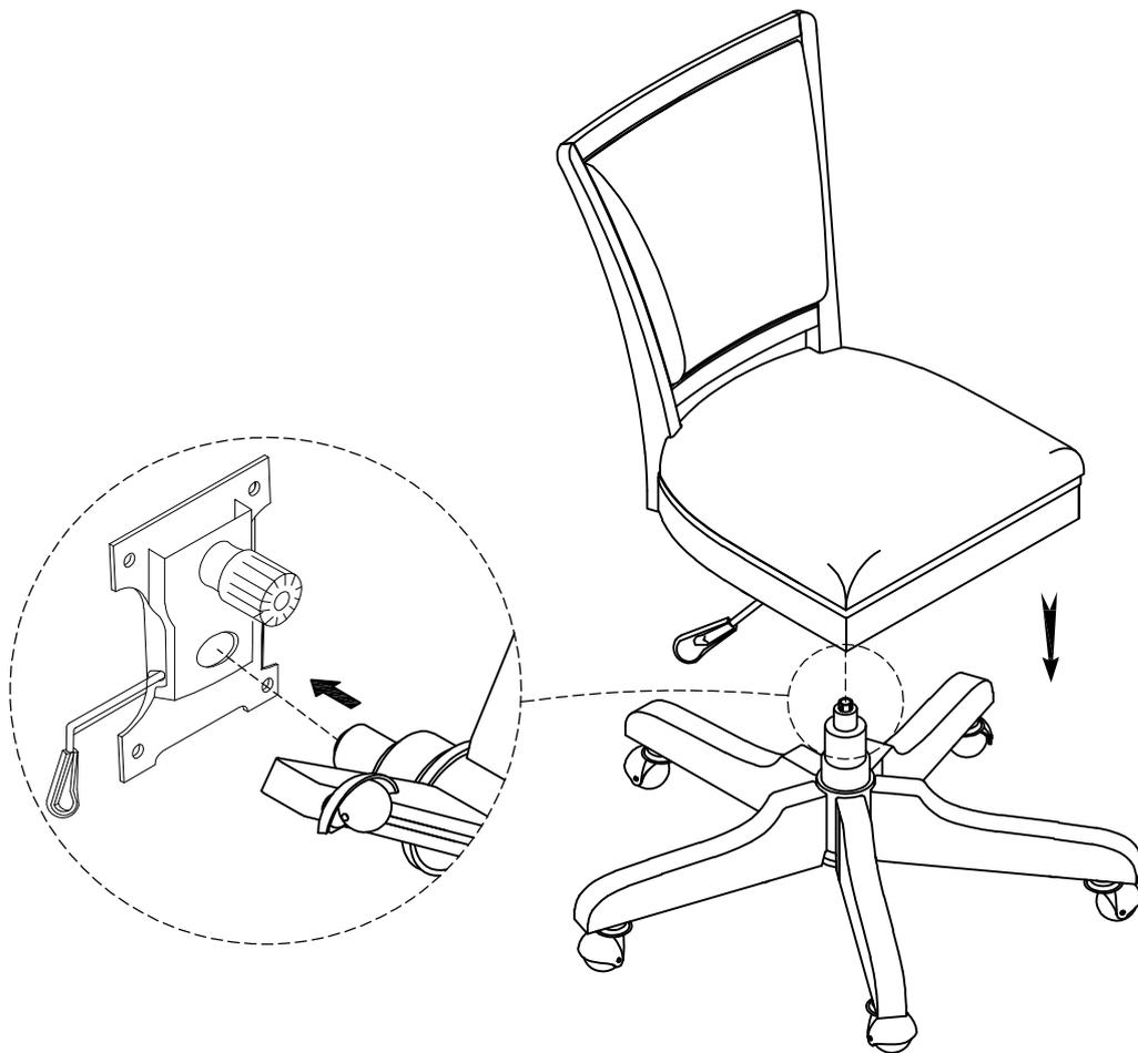
Note: To prevent possible damage to some types of flooring, never roll casters on unprotected hardwood or vinyl flooring. The lift mechanism is in a locked position for shipping. To unlock, pull straight out on the handle, and then the lift cylinder can be activated by lifting the handle.
