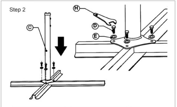
Attach the base stand (C) to the feet using four bolts (D) and four washers (E). Tighten the
