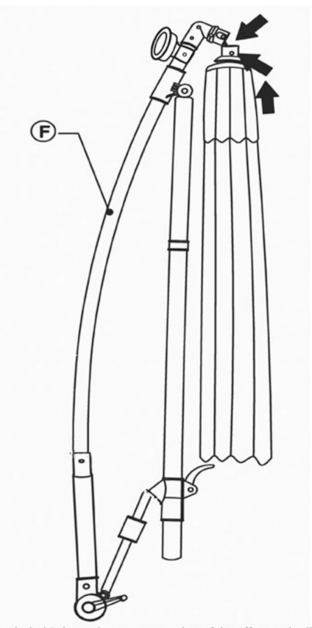
Connect the included Solar to the top support bar of the offset umbrella. This should twist and lock into place. Then connect the wiring before the next step.
