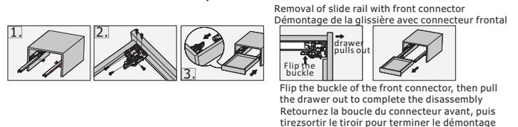
Removal of slide rail with front connector
