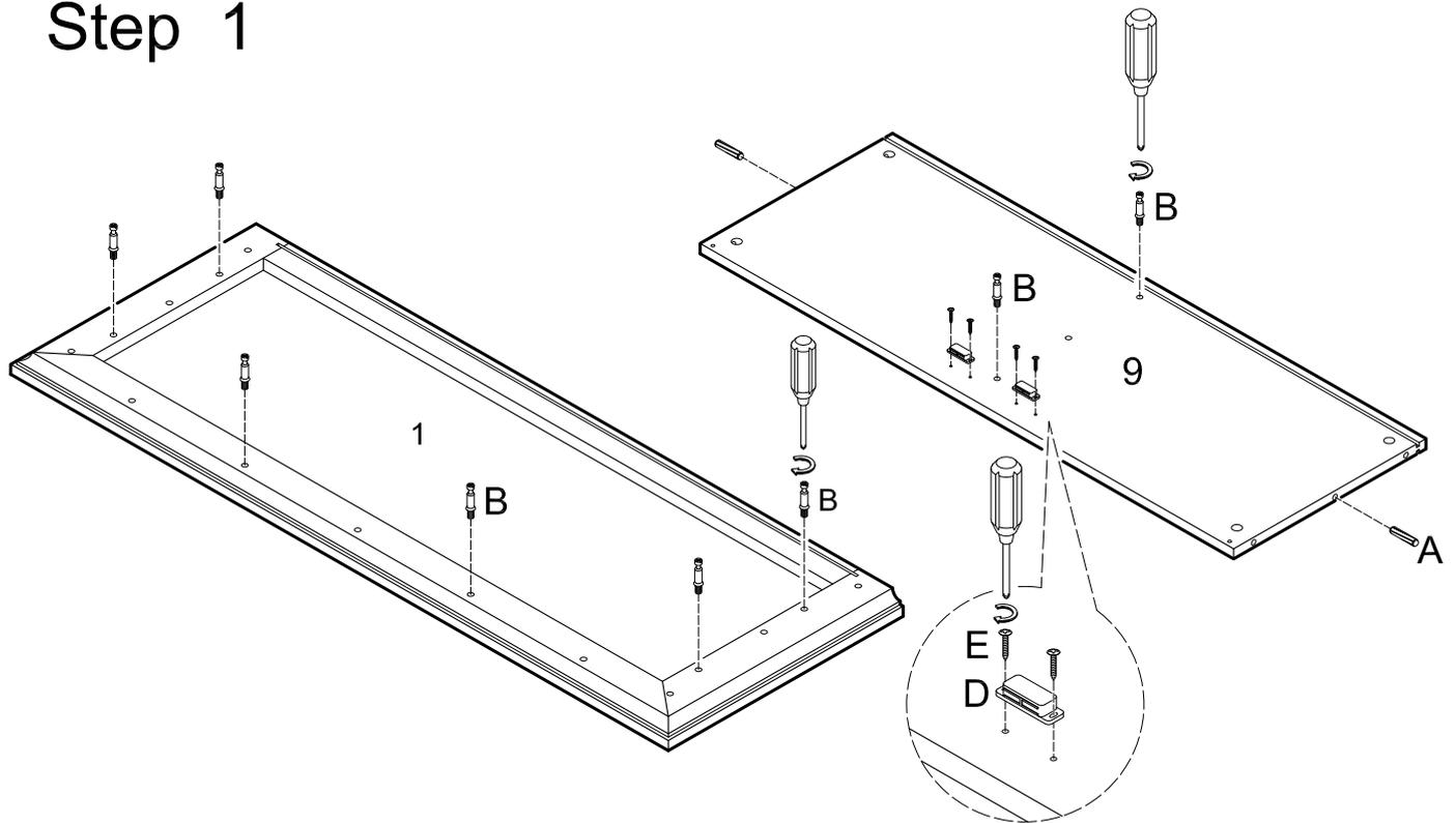
Screw cam bolts (B) into top panel (1) and shelf (9). Insert dowels (A) into shelf (9). Attach door stoppers (D) to shelf (9) using small screws (E).
