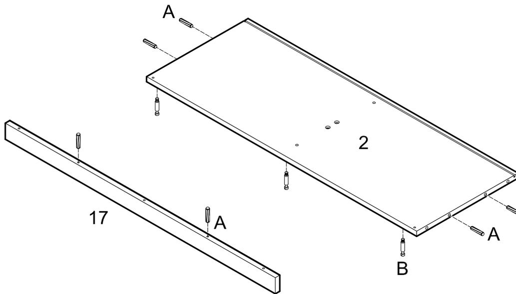
Screw cam bolts (B) into panel (2). Insert dowels (A) into panel (2) and slat (17).
