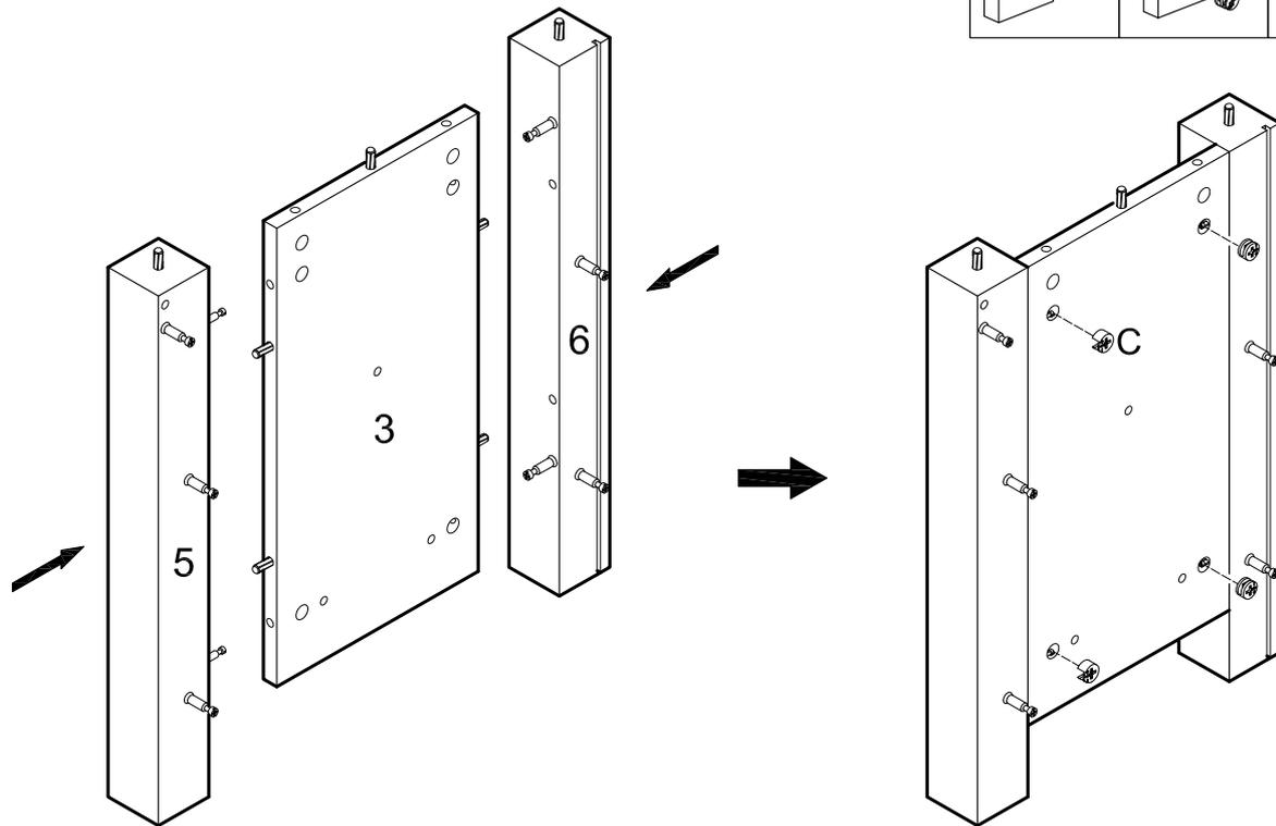
Attach legs (5,6) to panel (3) using cam bolts and dowels as guides. Insert cam locks (C) into panel (3) and tighten with a screwdriver.
