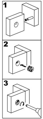
Insert cam locks (C) into the frame assembly. Attach top panel (1) to the frame assembly using cam bolts and dowels as guides. Tighten cam locks (C) with a screwdriver.
