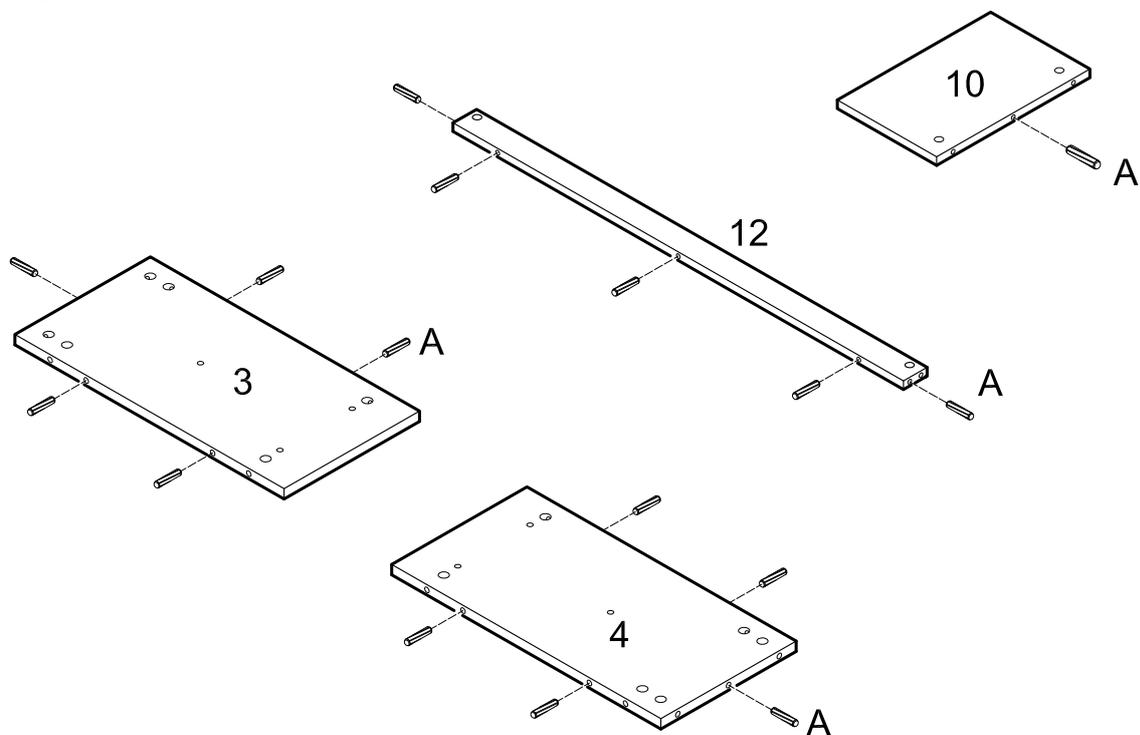
Insert dowels (A) into panels (3,4,10) and slat (12).
