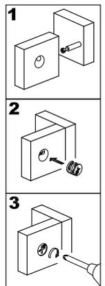
Insert cam locks (C) into panel (2), shelf (9) and slat (12). Attach the panel (4) assembly to panel (2), shelf (9) and slat (12) using cam bolts and dowels as guides. Tighten cam locks (C) with a screwdriver.
