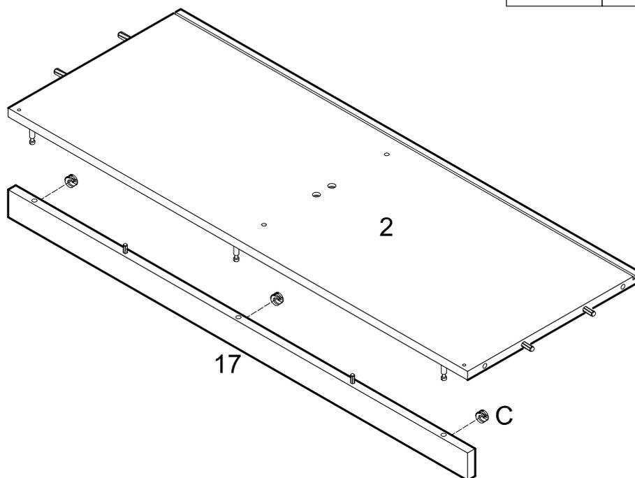
Attach slat (17) to panel (2) using cam bolts and dowels as guides. Insert cam locks (C) into slat (17) and tighten with a screwdriver.
