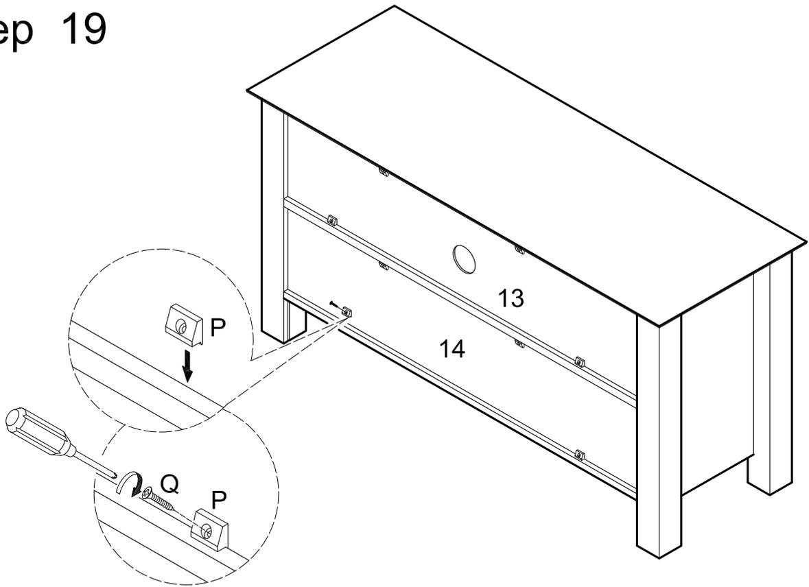
Secure back panels (13,14) using plastic wedges (P) and large screws (Q).
