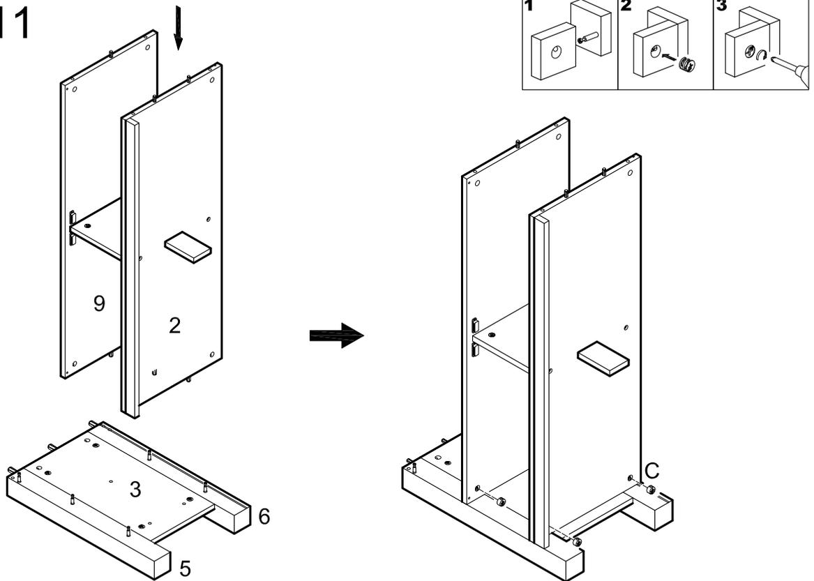
Attach the assembly from the previous step to the panel (3) assembly using cam bolts and dowels as guides. Insert cam locks (C) into panel (2) and shelf (9) and tighten with a screwdriver. Two cam locks will be inserted into panel (2) and into the shelf (9).
