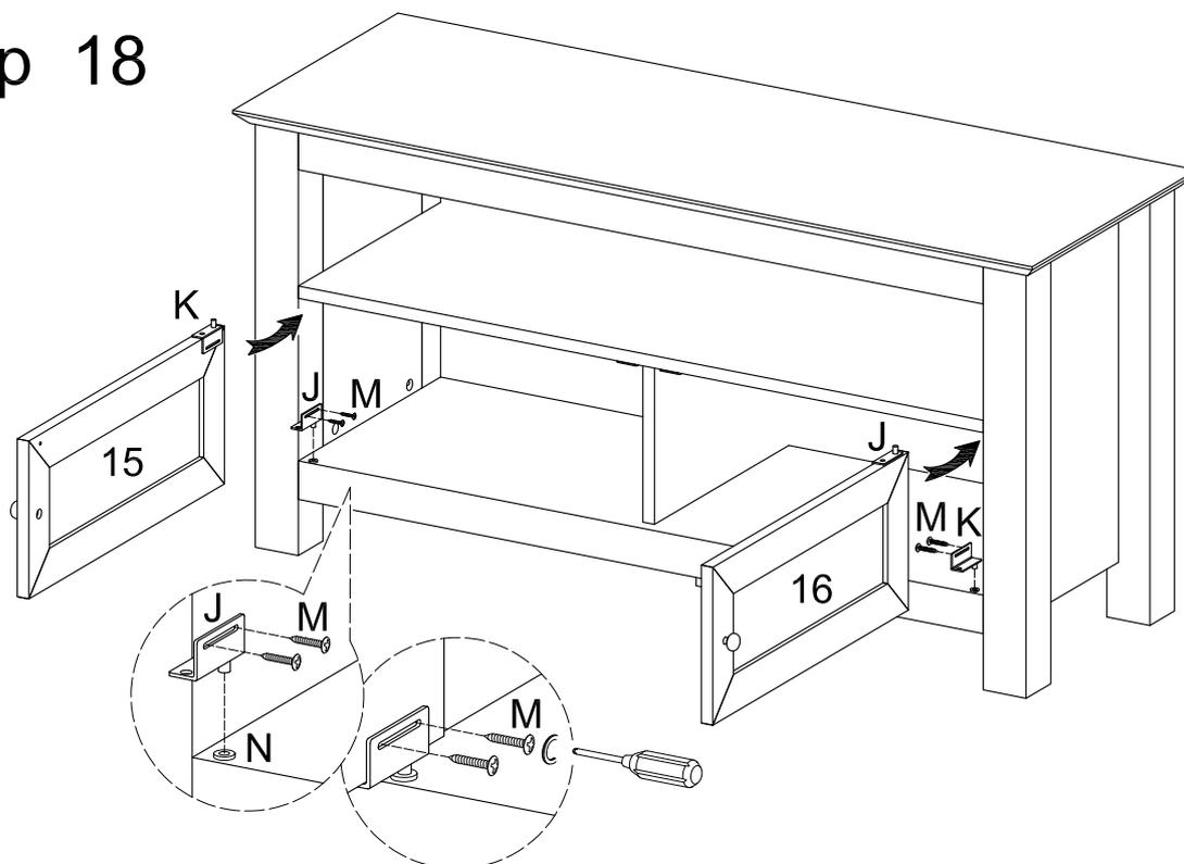
Insert door hinge (J) into left bottom plastic pivot (M). Slide door (15) into place. Attach door hinge (J) to door (15) using small screws (M). Insert door hinge (K) into right bottom plastic pivot (N). Slide door (16) into place. Attach door hinge (K) to door (16) using small screws (M).
