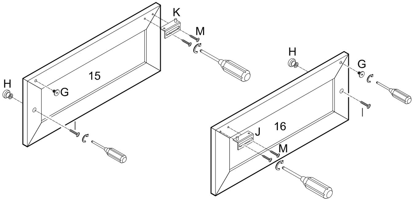
Attach handles (H) to doors (15,16) using medium bolts (I). Screw short bolts (G) into doors (15,16). Attach door hinge (K) to door (15) using small screws (M). Attach door hinge (J) to door (16) using small screws (M).
