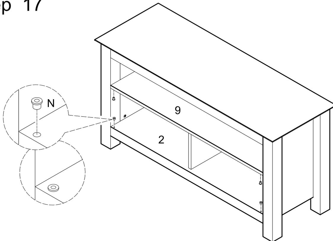
Insert plastic pivots (N) into panel (2).
