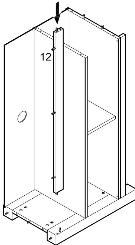
Attach slat (12) to the frame assembly using cam bolt and dowel as guides. Insert cam lock (C) into slat (12) and tighten with a screwdriver.
