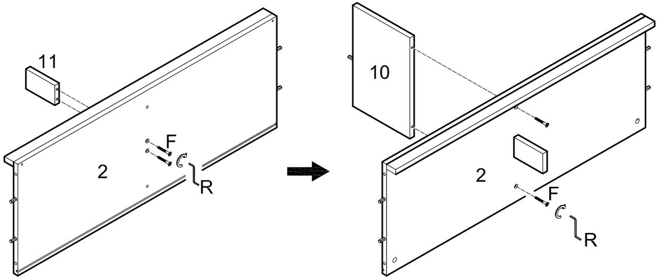
Attach support leg (11) to panel (2) using long bolts (F). Tighten long bolts (F) with wrench (R). Attach panel (10) to panel (2) using bolts (F). Tighten long bolts (F) with wrench (R).
