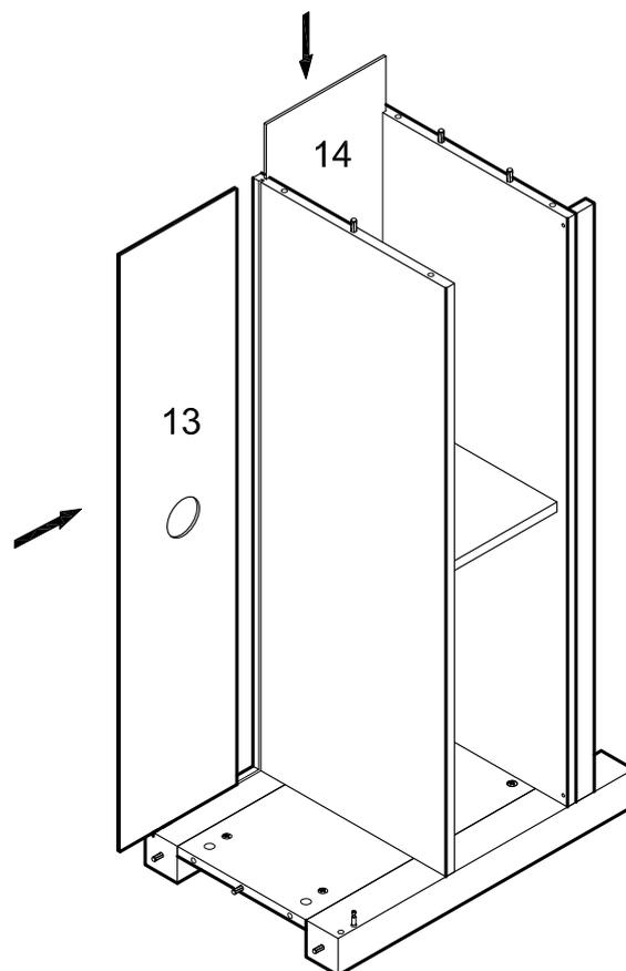
Carefully slide back panels (13,14) into place along the grooves at the back of the frame assembly.
