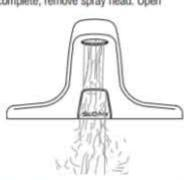
The OPTIMA Plus EBF-615 and EBF-650 Faucets are factory set to operate when hands are placed 4 to 5 inches (102 to 127 mm) from Sensor. This range should be satisfactory for most installations. If range adjustment is required, refer to the following range adjustment procedure.
