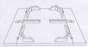
Fix the turned Leg to the corner of the apron with the Flat Washer, Spring Washer And Hex Nut using the Spanner to tighten it.
