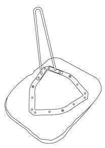
Line up one leg at a time to the holes in the mounting plate.
