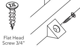
Screw in the brackets bottom with Flat Head Screw 3/4"
