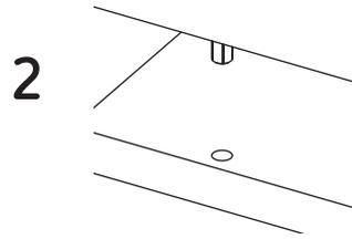
When joining two panels together, don't forget to gently hit the panels to adjust the joint.
