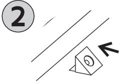
Insert the bottom supports between the groove and the bottom.
